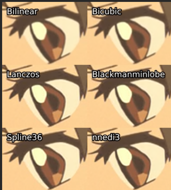
Figure 17: Comparison of resizers for upscaling. The source (Commie encode of Your Name (2016)) was cropped, then upscaled by a factor of 2.
