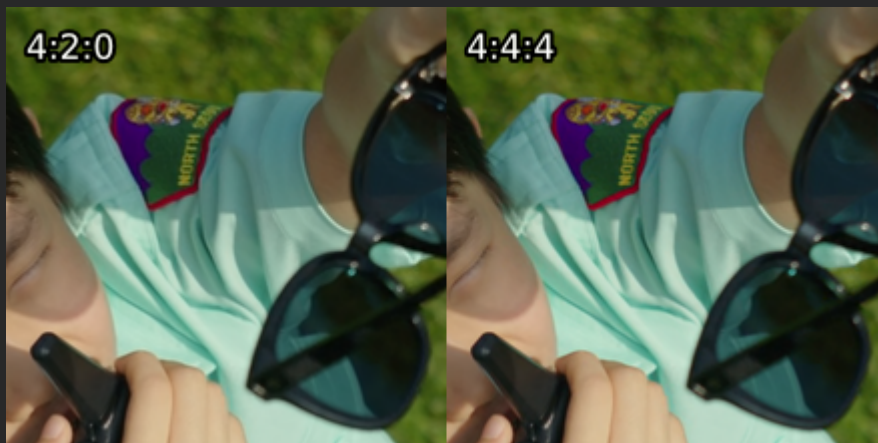
Figure 2: Parasite SDR UHD scaled to 1080p 4:2:0 compared to 4:4:4. Thanks go out to Hyer-rDoktyer for this example.
