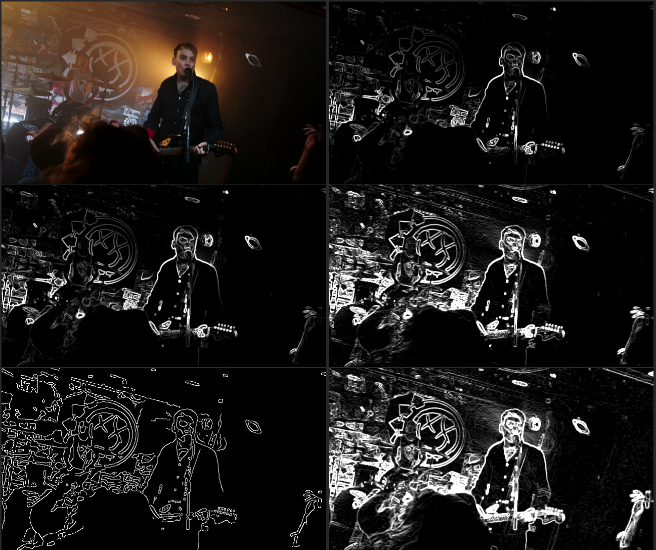
Figure 24: Comparison of different edgemasks. From top left to bottom right: source, Prewitt, Sobel, Kirsch, TCanny, and retinex_edgemask . All settings were left at their defaults.
