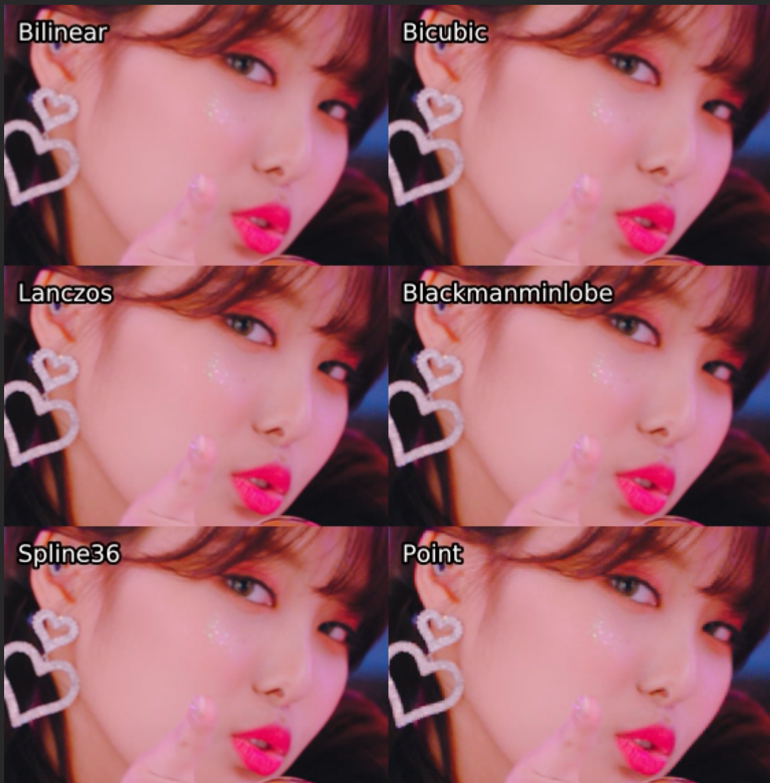
Figure 16: Comparison of resizers for downscaling. The source was downscaled from 1080p to 720p, then cropped. The parameters were all left at their defaults.
