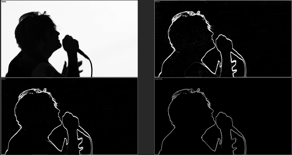
Figure 25: Comparison of the more accurate edgemasks. From top left to bottom right: source, retinex_edgemask , Kirsch, Sobel. Note that this is on a very poor quality source with terrible lighting, hence the difference between retinex and Kirsch masks is larger than usual.
